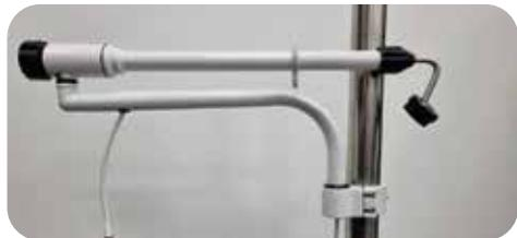
4. By tightening the fixator (by turning) the straight arm can move down and up for positioning.
