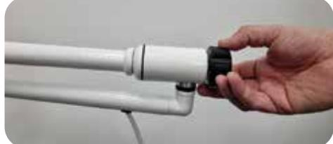
5. Mount the bleaching head by turning clockwise the conical fixator located on the telescopic arm. By turning the conical fixator located on the straight arm, the telescopic arm is firmly fixed.
